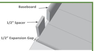
Leave at least 1/2" expansion spaces between flooring and ALL vertical objects (walls, cabinets, pipes, etc.) Large flooring runs may require additional expansion space. For floating floors, use transition moldings between rooms and in doorways. Undercut door jambs and casings to provide adequate expansion space. Do not screw or nail cabinetry or other permanent fixtures to a floating floor.
